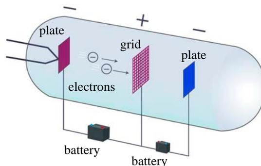
The Franck-Hertz experiment consisted of a tube of mercury gas, two plates, and a grid.
