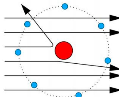
Placing a concentrated positive charge at the center of the atom explained the results of the experiment. Most of the alpha particles would travel straight, but some would bounce away.
