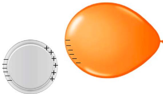
The negative charges on the balloon (right), forced the negative charges in the can (left) to move so that the positive charges were close to the balloon and the negative charges were far from the balloon.
