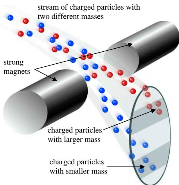
This is a very simplified drawing of a mass spectrograph. Since a magnetic field bends the path of charged particles based on their mass, you can use it to determine the mass of atoms or molecules.
