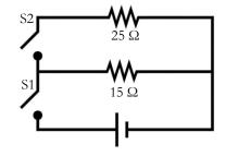
4. In the circuit on the right, suppose S1 is closed and S2 is open. If the battery shown is 9.0 volts, what is the current that flows from the battery?
