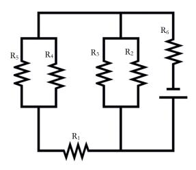
10. Which of the following fuses should be placed in the circuit shown on the right: 1A, 3 A, 5 A, 7 A, 9 A?
