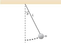
Think about the forces acting on the mass. Gravity is pulling down, and the tension in the string is pulling along the length of the string. That leads to the diagram on the right.
