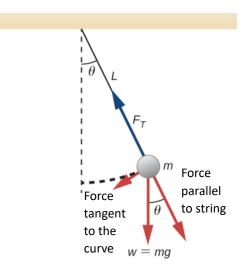
That means the force parallel to the string is adjacent to theta, which means it is  $mgcos(\theta)$ . That makes the other component (the one causing the acceleration)  $mgsin(\theta)$ .
