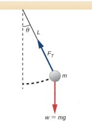
The gravitational force can be split into two perpendicular components: one parallel to the string, and one tangential to the curve along with the mass travels. That leads to the diagram on the right.
