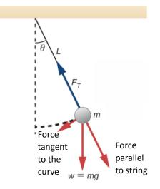
Notice that the weight is pulling straight down, which is in the direction of the dashed line that represents where the pendulum would hang if it weren't displaced. That means the angle between the weight and the force parallel to the string is also theta. That leads to the diagram on the right.
